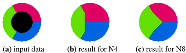
Fig. 9 inpainting . Depicted above are solutions (b, c) of synthetic instances of the inpainting problem (a). It can be seen that discretization artifacts due to the 4-neighborhood (b) are smaller than discretization artifacts due to the 8-neighborhood (c)
