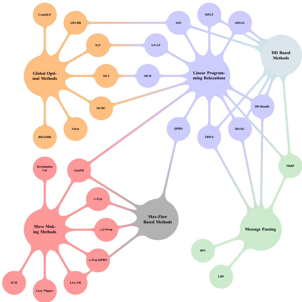
Fig. 4 The inference methods used in this benchmark can be roughly grouped into four classes. These are (1) methods based on linear programming , (2) methods providing global optimal solutions, which are often strongly related to linear programming, (3) methods based on move-making procedures which iteratively improves the labeling, and (4) methods based on message passing —often motivated by linear programming and variational optimization. Some methods make use of max-flow methods for fast optimization of binary (sub-)problems or based on the dual decomposition framework, which is also sketched in the diagram. A fifth class of methods are methods based on sampling , which are not covered in this study since they are rarely used
